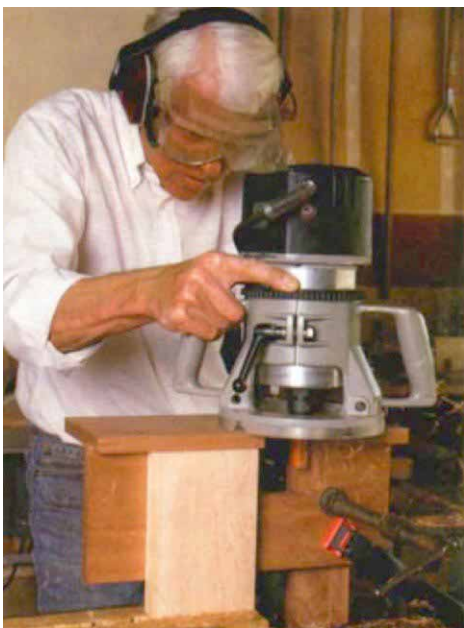
A good jig keeps the router in line. By controlling the line of cut, jigs make mistakes less likely.
